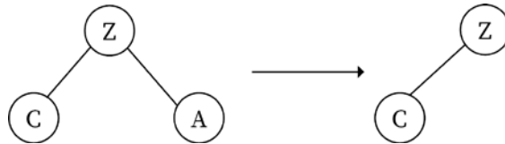
Figure 6.31: Deletion operation when deleting a node with no children
